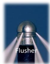
Three round nose double groove nozzles supply a smooth, compact design to easily navigate sewer pipe bends and turns for better handling and nozzle recovery. The Trio-F kit includes a penetrator, flusher, and a cornering nozzle. All nozzles combine thrusting power with a wide-angle spray for greater force in more challenging sewer situations. Pressure rated to 10,000 psi.
